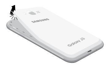
**Warning**: Do not bend or twist the back cover excessively. Doing so may damage the cover.
