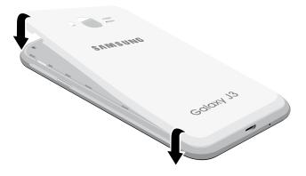
2. Press along the edge of the back cover until you have a secure seal.
