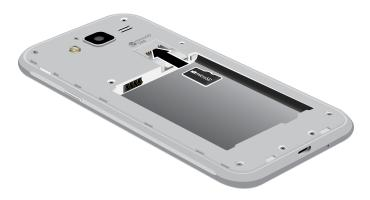
► Slide the memory card into the slot with the gold contacts facing down.
