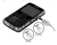
**Note:** This illustration shows both the correct method and the incorrect method for connecting the charger.
